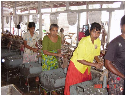
Hand paring process (waste reduced from 53 grams per nut to 45 grams per nut)
